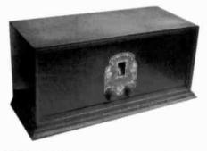
MURDOCK MODEL 65 – This "single dial tuning" receiver was manufactured by the Wm. J. Murdock Co. of Chelsea, Mass. It uses six Type 201-A tubes and a Type 71 output tube. In 1927, it sold for \$65. (Ray Chase – Plainfield, NJ)
