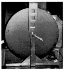
A different kind of home brew — a mechanical TV scanning disc and motor mounted on a wooden frame.
