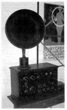
A Federal Model 61 driving a large Federal horn was playing during the open house using an ARBE-III battery eliminator.
