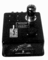
MAGNAVOX TYPE A1 – This 1-tube amplifier in a metal case sold for \$27.50 in 1923. The tube being used here is a rainbow Type 201-A. (Ross Mason – Mason City, IA)
