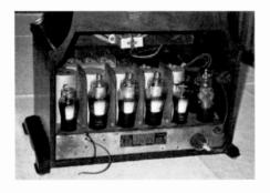
A rear view of the Model 93 showing the unusual 6-tube line-up on the rear edge of the chassis.
