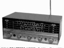
HALLICRAFTERS MODEL S-120 — This 1950s shortwave receiver has four bands and operates on AC/DC with the following tube types: 12BE6, 12BA6, 12AV6, 50C5, and a selenium rectifier. It has a ferrite loop for broadcast reception and a telescoping antenna for the shortwave bands. (Clark Trissell — Lincoln, NB)
