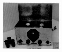
This rare 3-tube RIM Explorer, ca. 1930, uses (4) plug-in coils to cover the range from 1.5 to 17 MHz. Type 01-A tubes are used as a regenerative detector and two AF stages. RIM Radio Manufacturing was located in Brooklyn, N.Y.
