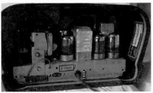
Figure 2. This photo of the back of the Philco Model 48-230 shows the chassis and tube placement.
