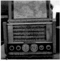
This Stromberg-Carlson Model AWP-8, an 8band, AC-DC & battery-operated portable included weather instruments and a world map.
