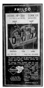
Figure 3. Label on the bottom of the Model 48-230 showing the chassis and tube layout.
