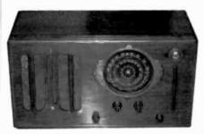
WESTINGHOUSE MODEL WR212 – This is a wood tabletop radio manufactured in 1936. Operation is AC with 8 tubes, including tuning eye. It also has both BC and SW bands. The tube types are 6K7, 6A8, 6F5, 6H6, 6F6 and 5Y3. (Michael Comer – Haslett. MI)
