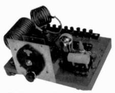
**HOME-BREW TRANSMITTER** – This 1-tube transmitter was recently constructed using 1928 vintage parts. It uses a Type 201-A tube. *(Ray Chase – Plainfield, NJ)*
