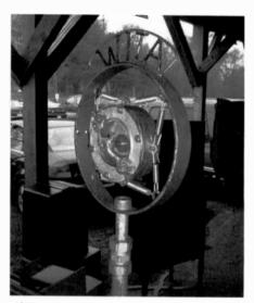
Radio Station WITA spring-type microphone.
