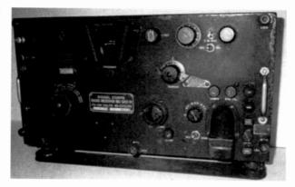
Figure 1. My Signal Corps radio receiver, Model BC-342.
