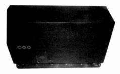
Figure 4. The restored cabinet after the sanding, priming, and painting operations.
