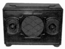
**GENERAL ELECTRIC MODEL BX** – This small, metal-cased radio was manufactured in 1932. The 4-tube chassis contains a voltage-dropping filament resistor. (*Jack LaVelle – Oak Forest, IL*)
