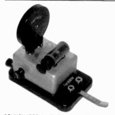
SCHUCHARDT ALLRATOR CRYSTAL SET – 1 looked for about 20 years for this most wanted set and finally bought it in 2002 in Sweden. Made in 1926 in Germany, it has condensator tuning (see the small lever), a plug-in detector from Selectit, and an Aeriola coil. It receives both long and short signals. (Erwin Macho – Vienna, Austria)
