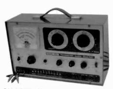
**B&K MODEL 960** – Your transistor radio not working? Use this B&K Model 960 transistor radio analyst to check it out. It provides eight separate DC voltages, an indivIdual transistor checker for in- or out-circuit testing, a VTVM, an output meter, and an RF/IF signal generator. (*Ray Chase – PlaInfield, NJ*)
