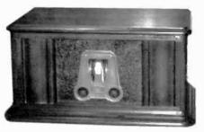
FRESHMAN MODEL F-1 EQUAPHASE – The production year for this tabletop set was 1927. This is a battery-operated radio using the following 6 tubes: (4) 201-A, and (1) each 200-A and 112. The instruction book pictures the Model F-4 (floor console) at a retail price of \$225, and the Model F-5 at \$250. Prices did not include the tubes. (Michael Comer – Haslett, MI)
