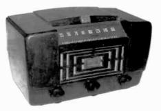
RCA VICTOR MODEL 66X11 – This brown plastic radio was sold in 1947. It has a 6-tube, AC/DC chassis and plays the broadcast band only. (Clark Trissell – Lincoln, NB)
