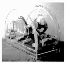
Figure 1. The Hypersonic neon radio with its transparent plastic cabinet, a feature which allowed the user to view the entire chassis components.
