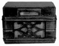
SILVERTONE MODEL 6406 – This 1940 wooden table radio has its chassis mounted upside down. It uses the following tubes: (1) each, Types 12B8, 12SK7, 12Q7, 35L6 and 35Z5. (Jack LaVelle – Oak Forrest, IL)
