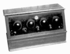
OZARKA 4-DIAL RECEIVER – Manufactured in 1924 by Ozarka, Inc., of Chicago, Illinois, this 4-dial battery receiver has 5 tubes with a battery box underneath. I have seen another version in the same cabinet with 4 tubes and an internal crystal detector. (Dave Crocker – Mashpee, MA)
