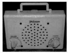
Figure 1. This Philmore Model TR201 uses two transistors in a reflex circuit for "multitransistor" performance.
