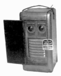
TOM THUMB MODEL ATTP – This portable radio was built in 1947 by the Automatic Radio Mfg. Co., Inc., of Boston, Mass. It is a 4-tube, AC/DC receiver, which has a rejuvenator to charge its batteries. (Wally Worth – Wollaston, MA)
