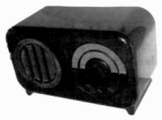
**EKCO MODEL AC85** – This 5-tube AC superhet receiver was manufactured in 1935 by E.K. Cole of Southend, U.K. The cabinet is moulded Bakelite. (Jim Taylor – Bournemouth, England)
