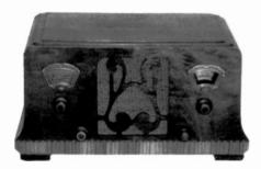
ZENITH MODEL 825 – Known as the "Twin Midget," this 7-tube, AC superheterodyne (BC + SW) has a large number of tubes for a table model and uses a separate oscillator tube. Progress in tube design allowed later models to combine the oscillator with the mixer/detector tube. The set has a relatively rare, series-tuned wave trap stated to "eliminate code interference" at the IF frequency. The cabinet has a unique wooden inlay running along the bottom. (Mike Grimes – Plano, TX)
