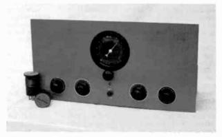
Figure 1. The front panel of the All-Star. Left to right, the four controls along the bottom: volume, antenna tuning, oscillator tuning, and tone. The airplane dial is for bandspread and provides a 0-100 logging scale over a 270 degree arc.
