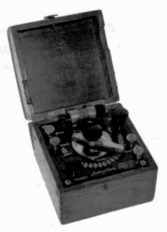
BRUCKNER "LUMOPHON" TYPE D CRYSTAL SET – Made in Nüremberg, Germany, this 1924 crystal set is maybe one of the best German-made sets. It has condenser and coil tuning and still has its original crystal detector. A highlight of my collection! (Erwin Macho – Vienna, Austria)
