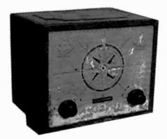
CROSLEY, MODEL UNKNOWN – This 2-tube radio was manufactured by the Crosley Radio Company, then owned by Avco. The simple circuit uses only two tubes: (1) Type 12A7 and (1) Type 6F7. The front of the radio is the speaker. Does anyone know the model number? (Geoff Shearer – Centreville, VA)
