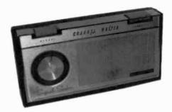
CHANNEL MASTER MODEL 6459 – This 10 transistor portable was manufactured in the late 1950's or early 1960's. It was marketed as the "Signal Seeker" which featured a motor in the rear that automatically tuned the stations by depressing the right-hand button. The left-hand button is for tuning manually. (Gerald Silver – Tamarac, FL)
