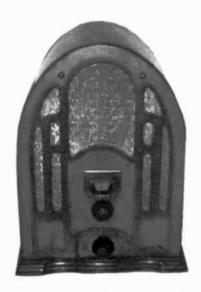
UNIVERSAL MODEL 42 – This cathedral was manufactured by the Universal Radio & Television Corp. It has a 4-tube TRF chassis using (2) Type 24s for RF amps, (1) Type 47 for audio and (1) Type 80 as a rectifier. It sold for \$160 in 1932. (Jerry Wieland – Hoffman Estates, IL)
