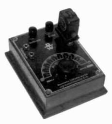
**DTW TYPE D.E. 3** – This German Crystal set has seven different plug-in crystal units. It was manufactured in 1926 by Deutsche Teleponwerke and Kabelindustrie A-G. The front panel is alumlnum. (Erwin Macho – Vienna, Austria)
