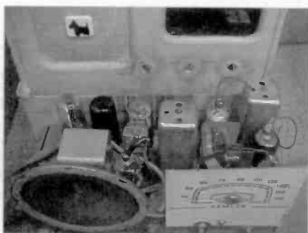
Here is the typical chassis of the "picnic portable" radios, this one for the Remler Scottie 93.
