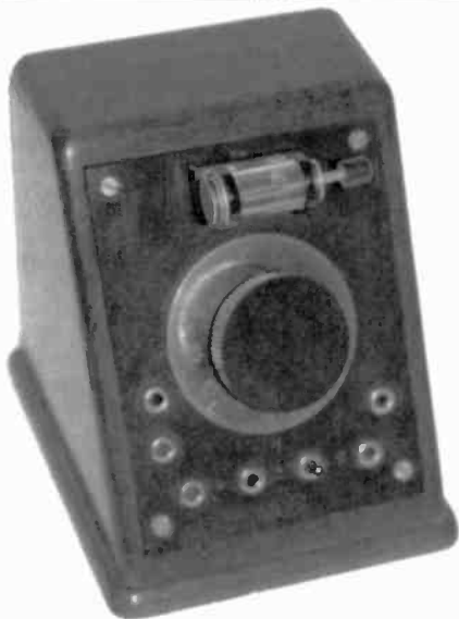
AGA CRYSTAL SET – This 1926 crystal set was made in Sweden. It has variometer tuning inside its wooden case and jacks for two headphones. ( Erwin Macho – Vienna, Austria )
