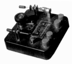
WESTINGHOUSE DB DETECTOR – This 1922 dual crystal detector has a switch to allow the operator to choose the type of detector he wants either the perikon (mineral-to-mineral) type or the catwhisker/galena type. A phone condenser is mounted under the Bakelite frame. (*Dave Crocker* – *Mashpee, MA*)
