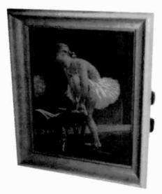
PICTURE FRAME MODEL 844B – This framed painting of a young ballerina and her dog is actually a radio. It was manufactured by Bell Products, Futura Division, in the 1950s. The radio controls can be seen on the right side. The dial shows the "CD" symbol pertaining to "Civil Defense." (Norman Landis – St. Louis, MO)
