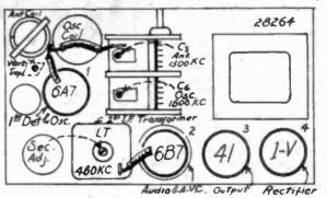
Figure 4: Chassis layout for the RCA 4-T receiver.
