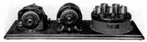
Figure 1. The Atwater Kent Duplex Model 8 receiver.
