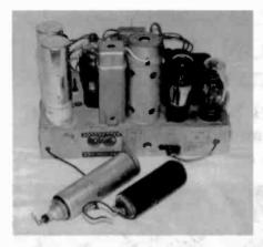
Figure 2. The compact chassis of this "4-tuber" is shown with new filter capacitors in place. The two capacitors in front of the chassis are the bad units.
