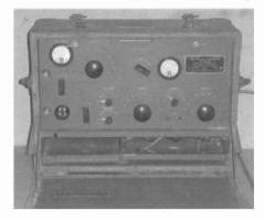
Early 1930 U.S. Army field radio BC-157. The transmitter uses one tube; the receiver, three tubes. The frequency range of this equipment is about 3800 Kc to 4200 Kc, and it uses CW (Morse code) only.
