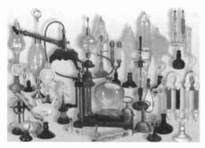
A dazzling display of early Crookes and Geissler tubes and vacuum pumps.
