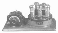
Two of the sixteen Atwater Kent breadboards are shown here. Above is a crystal set and, shown below, a Model 5.
