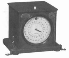
Early telegraph equipment is represented by Bréguet's ABC (or dial) telegraph from 1850-1870. The transmitter is left and the receiver, right.
