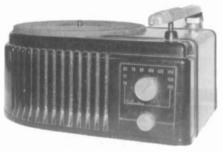
SILVERTONE MODEL 7070 – This radio/phonograph combination, manufactured in 1949, is housed in a Bakelite cabinet. The 5-tube, AM band radio uses one each of the following tubes: 14A7/12B7, 7C6, 14Q7, 50A5, and 35Y4. The phonograph plays 78 rpm records only. (Clark Trissell – Lincoln, NB)
