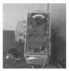
Front view of IM-37A RFI (Radio Frequency Interference) meter that is part of the Navy's PRM-1 system. The receiver tunes from 150 Kc to 25 Mc and is used to evaluate noise and interference levels at communications sites and locations. Provision is made to record the receiver output on strip charts for later analysis.
