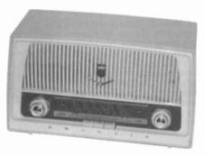
GRUNDIG TYPE 87 – This early German, 1960s, plastic-cased, tube-type radio has the design of the earlier wood-cabinet Grundig sets. (Erwin Macho – Vienna, Austria)
