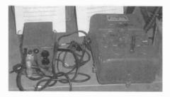
The rare Eureka beacon set used during World War II. The gear operates in the UHF band between the 214 to 234 Mc range.
