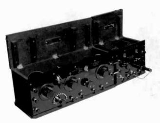
KENNEDY TYPE 281 AND TYPE 521 – This 2-unit combination set Is made up of a Kennedy Type 281 1-tube receiver and a Type 521 2-tube amplifier. The set was manufactured In 1921 by the Colin B. Kennedy Co. of St. Louis and San Francisco. The receiver has regenerative circuitry and tunes from 180 to 620 meters. (Dave Crocker – Mash-pee, MA)
