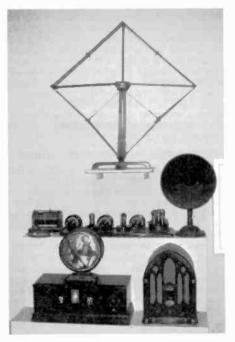
Figure 2. Among the other items in the exhibit was this display of a loop antenna, a crystal set, a breadboard, a horn speaker, a battery set, and a GE cathedral.
