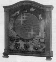
PHILLIPS MODEL UNKNOWN – This 4-tube, local-station receiver is housed in a wooden cabinet with an ornate pagoda design. It was manufactured in 1930-1931. It also came in a cathedral-style cabinet made of Arborlite. (Jim Taylor – Bournemouth, England.
