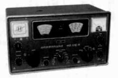
HAMMARLUND MODEL HQ-110A – This metalcased radio is a quality shortwave receiver. It tunes from 160 to 6 meters. The circuit uses the following tubes: (2) 6BZ6, 6BE6, 12AX7, 6BA6, 6AZ8, 6BJ7, 6AQ5, 6C4, 5U4, and 0B2 regulator. (Clark Trissell – Lincoln, NB)
