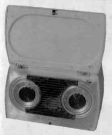
MOTOROLA MODEL 5A9M – This portable, 5tube AC/DC radio was sold in 1948. The cabinet is metal, and the set plays when the flip-up front cover is opened. The dial on the left is for volume only, while the one on the right is for tuning the broadcast band. (*Clark Trissell – Lincoln, NB*)
