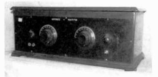
Figure 1. This front panel view of the Haynes-Griffin Superhet shows the two main tuning control dials, the two rheostat controls beside the two dials, the off-on switch (lower right), and the two phone jacks at the far left.
