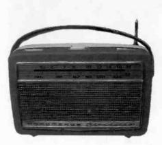
NORDMENDE STRADELLA – This 1962, 6-transistor, AM/FM radio was made in Germany. Its allwood case is covered with a grained leatherette. It has a telescoping antenna and the power cable terminals clip on to a 6-volt battery. (Francis H. Yonker – State College, PA)
