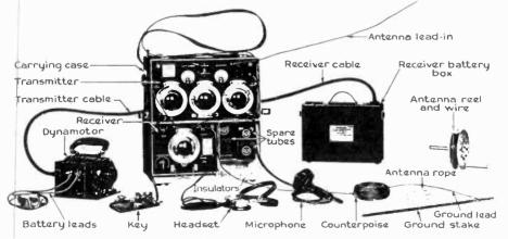
Figure 5. The complete Coast Guard Model T-22 system, which includes the transmitter, receiver, generator, battery box and all components. (From GE documentation dated 7/14/32)
