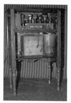
Figure 5. This rear view shows the chassis and the enclosed speaker compartment.
