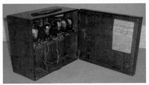
Figure 4. The Marconi Model 55 receiver shown with the back cover open to expose the tubes and the instruction and calibration chart attached to the back cover lid.
