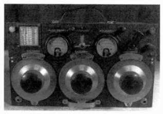
Figure 1. The 5-watt Coast Guard Model T-22 (RT-80A) portable transmitter unit.
