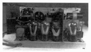
Figure 2. The Model T-22 transmitter with its rear cover removed showing the Type 112-A 4-tube line-up.
