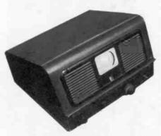
**PILOT MODEL TV-37** – This 1949 television set, with synchronous tuning, was the first TV to sell below \$100. Its price was just \$99. The picture tube is only 3" in diameter (3KP4). (Dave Crocker – Mashpee, MA
