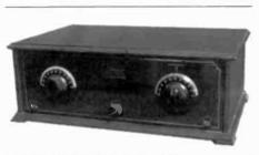
SILVER-MARSHALL TYPE 630 - This 1928 "Shielded Six" uses five Type 201 tubes, plus a Type 112, has four tuned stages, three of which are in separate shielded compartments. It was advertised as an AC set when used with a companion battery eliminator. (Ray Chase - Plainfield, NJ)
