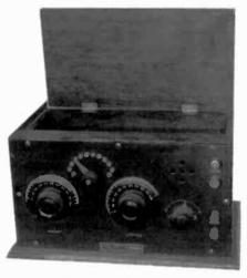
AMES TYPE DCR - This 1-tube receiver was made by the Pickard Radio Corp. of New York. A matching amplifier was also available. (Merrill Bancroft - Townsend, MA)
