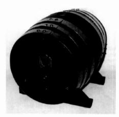
Figure 1. Radiokeg Model RK-S-5 recently restored using a diode as a replacement for a resistance line cord.
