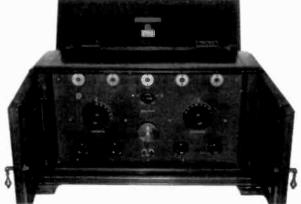
GECOPHONE BC2050 – This 1924 5-tube battery set was the company's top-of-the-line receiver. It is considered rare, as most British radios of the early 1920s were 2- or 3-tube sets. All British radio manufacturers had to pay a rather high royalty to Marconi for each tube in the circuit. (Jim Taylor – Boumemouth, England)
