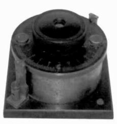
TUNING CAPACITOR, MANUFACTURER UNKNOWN – This variable air capacitor measures  $4^1/2^n \times 3^1/2^n$ . It has 50 aluminum plates that are  $3^3/2^n$  round. The Bakelite dial sits on a brass case with a Bakelite base. (Paul Recupero – Portsmouth, RI)
