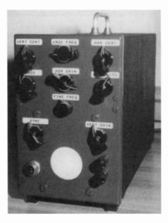
Figure 5. The completed oscilloscope with its repainted front panel and new legends.
