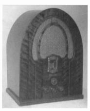
Figure 1. My Philco Model 89B from 1933 is a 4-knob version that tunes both the Broadcast and SW bands.
