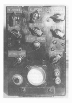
Figure 1. The home-brew 2" oscilloscope as acquired.
