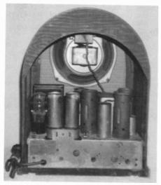
Figure 2. This rear view of the Philco Model 60 shows the compact arrangement of the radio's components.
