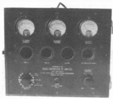
RCA TUBE TESTER – This is an early 1920s tube tester made only for RCA radio dealers and service centers and not sold to the public. It is battery-operated and tested RCA tubes, such as WD-11, WD-12, 199, 200, and 201A. (Ross Mason – Mason City, IA)
