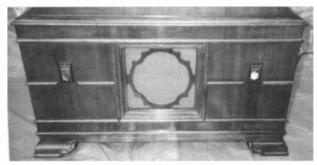
Figure 1. Front view of the Kennedy Model 26 showing the only visible control — the tiny radio dial at the right.
