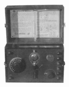
HOME TYPE CT RECEIVER – This unique receiver was sold in 1922 by the Home Radio Corp. at 100 Madison Aveue in New York City. The operator could either use the catwhisker crystal detector viewed behind a glassed-in dome (above center), or flip the center bottom switch to the one internal tube for detection. (Merrill Bancroft – Townsend, MA)
