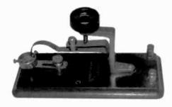
A.W. BOWMAN DETECTOR – This very sensitive crystal detector was manufactured by A.W. Bowman & Co. of Cambridge, Mass. (Merrill Bancroft – Townsend, MA)
