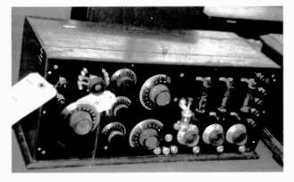
This unusual and early receiver is equipped with 3 Meyers type, panelmounted tubes and an enclosed crystal detector. It sold for \$1,100.
