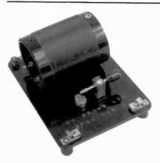
W.W. GRANT LIMITED CRYSTAL SET – This receiver was fixed at the wavelength of the W.W. Grant broadcasting station in Calgary, AB, CFCN, at 440 meters. The station operated from 1922 to 1927, after which it was sold to cover the cost of a court judgment. More details about Grant are in the August 1992 issue of the OTB. (Bob Murray – Winnipeq, MB, Canada)
