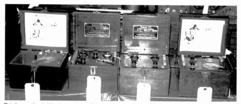
This lineup of early Westinghouse and RCA Radiolas include, left to right, the Aeriola Jr., a crystal set; the Radiola RS, a 2-tube receiver; the Radiola AC, a 2-tube amplifier; and the Aeriola Sr., a 1-tube receiver.
