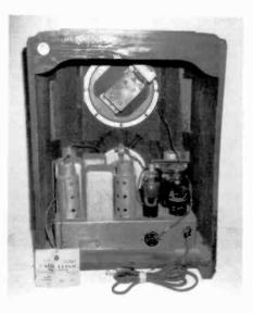
Figure 2. The condition of the converted chassis equals that of the cabinet. The added Type 5Y3 rectifier tube is located on the far right of the chassis.
