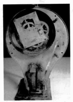
Figure 2. Rear view of the Bristol recording voltmeter, shown with the back cover removed to show the Seth Thomas clock movement set at an angle.
