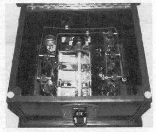
Figure 2. An interior view of the set shows the 3-section tuning capacitor, the five Kellogg tubes and the Type 71A tube. The two pieces of U-shaped bus bar make the filament connections to the snap-on filament connectors used with the Kellogg tubes. The volume control is located at the rear of the chassis.
