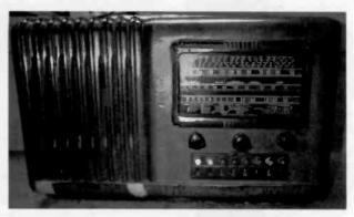
Figure 1. The 8-tube, 3-band radio in its "as found" state. Note the missing veneer on the lower edge of the cabinet.
