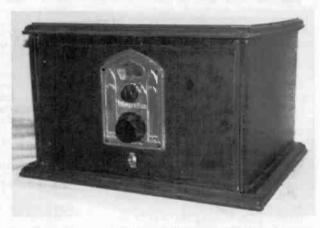
Figure 1. A front view of the restored Wurlitzer "Navaho" Model. The large knob is the funing control and the small knob controls volume. The toggle switch below the escutcheon is the on-off switch.
