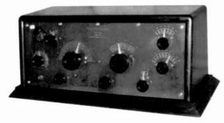
ZENITH 1R - This 1-tube receiver was manufactured by the Chicago Radio Laboratory in 1922. If has Serial Number 2369 and is licensed under the Armstrong U.S. patent of October 6, 1914. The front panel is made of hard rubber with a red coloration. The rear has a pull-down door to access the chassis. (Wally Worth - Wollaston, MA)
