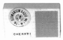
CHERRY CRYSTAL RADIO – This tiny, plastic, germanium crystal radio was manufactured in the 1960s. Notice the small compass built into the center of the tuning dial. (Erwin Macho – Vienna, Austria)
