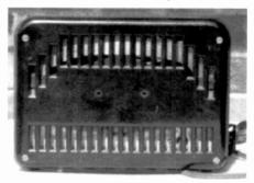
Figure 2. While many AC/DC radios from the 1940s used cardboard back covers, the Lyric used a Bakelite cover.
