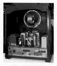
Figure 2. This rear view of the Model 127 shows its orderly component and tube layout.
