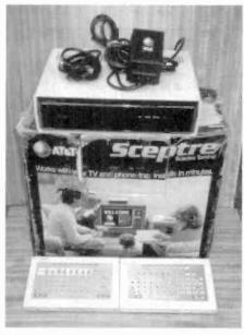
Figure 1. The Sceptre Videotex Terminal, power supply, cables, and keyboards. The AT&T keyboard is on the left; Western Electric on the right.
