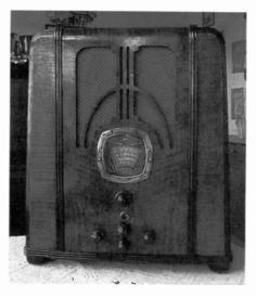
Figure 1. The front view of the Patterson Model 127. This allwave radio covers the frequency range of 545 kHz to 20 MHz.
