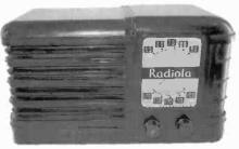
RADIOLA MODEL 500 – Manufactured by RCA Victor, this *circa* 1941 midget radio has a 5-tube chassis in a walnut Bakelite cabinet. The tube complement is Types 12SA7, 12SK7, 12SQ7, 35Z5, and 50L6. (Jim Ligouri – Atkinson, NH)
