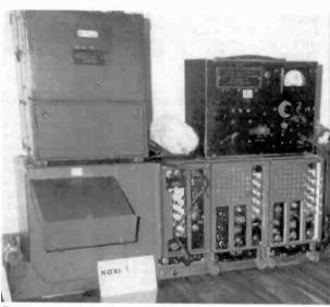
Two pieces of test equipment are sitting on top of this SCR-608 VHF FM set. The transmitters and receivers operated in the band from 20 to 40 MHz and were installed in a number of army tanks. The open drawer at the left contains extra crystals for frequency changes. Phil Epstein brought the set from Minneapolis for display.
