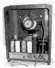
Figure 3. The interior of the Atwater Kent Model 545 after its restoration.
