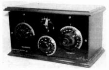
Figure 1. The Chelsea Model 104, a 1-tube set manufactured in 1922.
