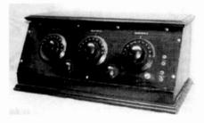
Figure 3. A front view of the 5-tube Chelsea Super-Five, manufactured in 1925.
