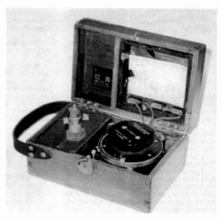
Figure 2. A Marconi Wireless Telegraph Co. Wavemeter in its case after restoration by the author.
