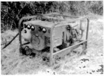
Over 150 feet of cable separates the 4-cylinder gasoline driven generator set and the TRC-75 installation operated by Dave Ross.
