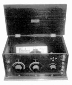
**OVERLAND RECEIVER** – This 1-tube receiver was manufactured by the Overland Radio Corp. of New York City. (Merrill Bancroft – Townsend, MA)
