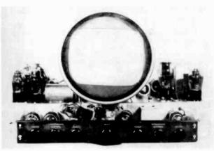
Figure 4. This front view of the chassis shows the set up controls described in the text and the 10" picture tube.
