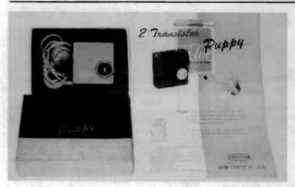
"PUPPY" TRANSISTOR RADIO - Manufactured by the Japan Lisistor Co., Ltd., this 2-transistor receiver was advertised as the smallest transistor radio in the world, weighing a mere 40 grams. Inside is a flat-type mercury battery. The plastic case came in either red, green, or tan, and it is shown here in its presentation box containing the earphone. (Erwin Macho - Vienna, Austria)
