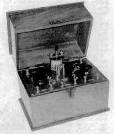
REFLEX CRYSTAL RADIO - Manufactured in the early 1920s by the Reflex Radio Co., this British receiver has a glass-enclosed crystal detector. The hardware is all gold-plated. (Jim Taylor - Bournemouth, England)
