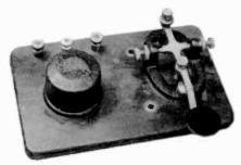
SIGNAL ELECTRIC PRACTICE SET – Used to practice the art of sending Morse code, this key-on-board set was manufactured by the Signal Electric Manufacturing Co. It consists of a brass and cast-metal straight key and a buzzer mounted on a walnut board with turned brass binding posts. (Dave Crocker – Mashpee, MA)
