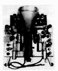
Figure 3. This chassis from the export model used 6-pin and 7-pin ST style glass tubes as well as octal based tubes. It is thought to contain only the deflection circuitry.
