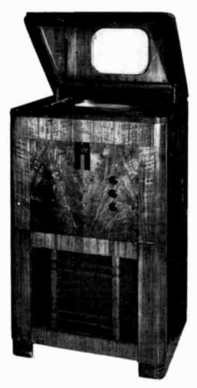
Figure 1. This RCA TV set is believed to be an engineering model from about 1935. Its cabinet styling and mirror-in-the lid picture are similar to RCA's Model TRK-12.
