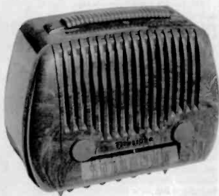
FIRESTONE MODEL 4-C-16 – This 1950 portable is a 4-tube radio using Types 1R5, 1U4, 1U5 and 3V4 tubes. It operates on either batteries or AC power. The lightweight case is a pretty, swirled brown plastic. ( Cyril G. Brennan – Pike Road, AL )
