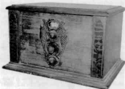
ALL-AMERICAN MOHAWK NAVAJO – This 1926 battery-operated receiver uses 6 tubes and features 1-dial tuning. The Mohawk series had early American names; hence, the arrowhead-shaped escutcheon. ( Wally Worth – Wollaston, MA )
