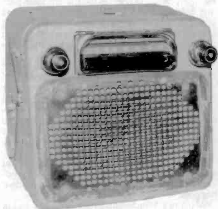
DELCO MODEL 987682 – This early 1950s car radio was made by the Delco Radio Division of General Motors Corp. for use in its own automobiles. Called the "Selectronic" radio, it has the standard 5 push buttons. ( Clark Trissell – Lincoln, NE )
