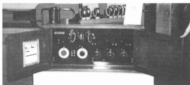
Figure 5. This early Dutch radio uses plug-in coils.
