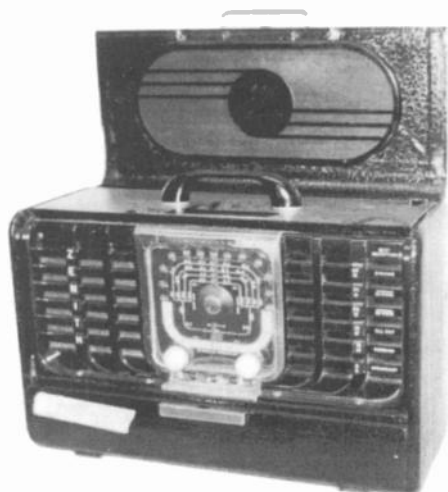
ZENITH MODEL 8G605 – This 1942 Trans-Oceanic multiband receiver has 8 tubes and the familiar Wavemagnet antenna. It was just one of the many shortwave Trans-Oceanics made by Zenith. ( Wally Worth – Wollaston, MA )
