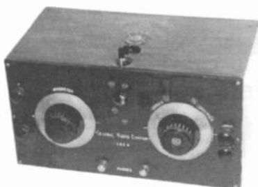
GENERAL RADIO TYPE GRC4 – This crystal receiver, manufactured in 1922, has the British G.P.O. Number 132. It has a small window opening in the front panel to view the position of the catwhisker on the crystal. One opening in the top is for adjusting the detector arm, and the opening behind it is for illuminating the detector. This great set has an important place in my collection. ( Erwin Macho – Vienna, Austria )
