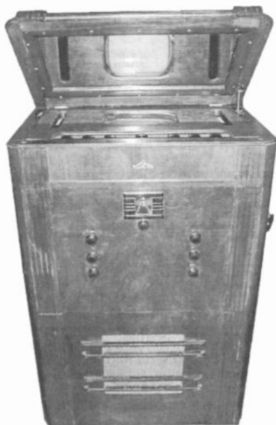
RCA VICTOR FIELD TEST TV MODEL RR-359 – This 9" TV console was made in 1936 for experimental use by RCA-NBC engineers. In 1937/1938, many were "recycled" to make 12" sets, most of which are in museums. This set won "Best of Show" and "People's Choice" at the March 2001, Charlotte, North Carolina, CC-AWA meet. It works quite well and has a greenish hued phosphor. ( Nat Pendleton – Columbia, SC )
