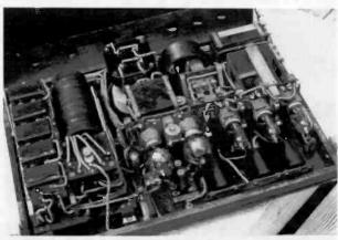
Figure 2. The interior of the CW-938. The front panel and chassis are unlatched and lowered to show the heavy construction and tight constraints of the component. You can see the layout of the two Type VT-2 and three Type VT-1 tubes.
