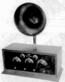
MURDOCK MODEL 200 - This 5-tube receiver, manufactured by the William J. Murdock Co. of Chelsea, Mass., sold for \$100 in 1924. Its unique feature is that the price included a Murdock adjustable horn speaker that fits into the receiver's top cover lid. (Ross Mason - Mason City, IA)
