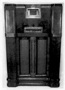
Figure 4. This Alrline Model 62-403 has an unusual grille cloth configuration. In addition to the flat surfaced grille cloth at the rear, this set utilizes a curved grille cloth in its center grille.
