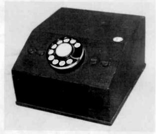
Figure 1. The unusual instrument that I first thought to be a telephone. From left to right, the push buttons on each side of the telephone dial are marked "ON," "OFF," "SOFT" and "LOUD."
