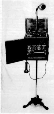
This 1906 Collins spark transmitter telephone combination uses an induction coil.
