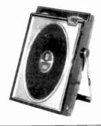
ZENITH ROYAL 500H - This early pocket radio uses 8 transistors for reception and 4 Type AA batteries for power. (Clark Trissell - Lincoln, NE)
