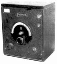
PHILMORE RADIO - Although the Philmore Company is well known for producing many types of crystal sets and crystal detectors, it also made this 2-tube receiver in 1925. (Wally Worth - Wollaston, MA)
