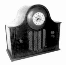
TOWER HOUSE RADIO – This cathedral-style radio, ca. 1931, is housed in a mahogany cabinet. The metal label on the rear of the cabinet reads, "Tower House Radio, H.M Tower Corporation, Distributor American Bosch Radio, Boston-Springfield-New Haven." This radio has 5 tubes, and the clock was made by General Electric. (Jim Ligouri – Atkinson, NH)
