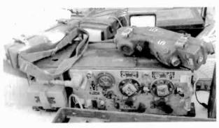
The large unit is a Wireless Set #19 that was made in the U.S. and sent to Russia during WWII for use in tanks.
