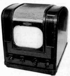
ELECTROMATIC TV, MODEL UNKNOWN — No model number or manufacturer's address appears on this late 1940s TV. It has a 10" CRT and tunes from Channel 2 to Channel 13. The speaker is at the top of the cabinet. Does anyone have more information on this set? ( Ross Mason — Mason City, IA)
