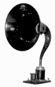
MAGNAVOX TYPE R2 MODEL B HORN SPEAKER - This hom speaker came with the Magnavox Type AC-2, Model C amplifier. (Joseph G. Jackson - Macon, GA)
