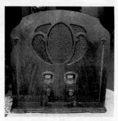
Figure 1. A front view of the 8-tube Kolster Model K-165 with the typical oval pattern grille favored by Kolster.
