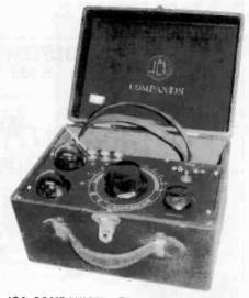
ICA COMPANION - This leatherette portable looks as if it should be a battery set, but it is actually an AC portable with two Type 27 Arcturus blue tubes. It measures 11" wide x 65/e" tall. (Wally Worth - Wollaston, MA)
