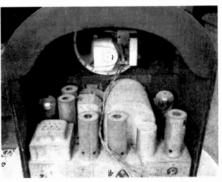
Figure 2. This rear view of the Kolster K-165 shows the chassis layout. The dome-shaped shield on the right covers the bandswitch. The smaller shield at the left covers the tuning capacitor.
