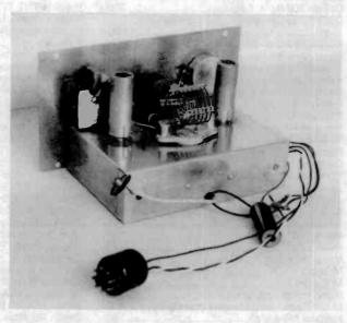
Figure 2. The rear view of the restored receiver shows its neat layout and its 80-meter coil.
