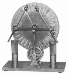
WHIMHURST MACHINE, MODEL UNKNOWN - This device, date unknown, was manufactured by Philip Harris Co. in Birmingham, England. The metal components are brass. Spark discharges of 5" to 6" are readily obtained. (Joseph G. Jackson - Macon, GA)
