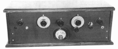
Figure 7. This 3-tube BC/SW home brew performed so well that the author restored it rather than strip it for parts.
