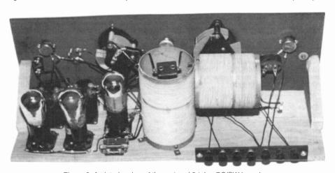
Figure 8. An interior view of the restored 3-tube, BC/SW homebrew.
