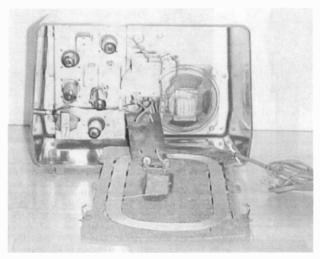
Figure 3. A top view of the chassis and loop antenna after the chassis was cleaned and repaired.
