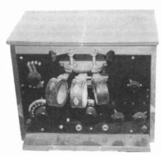
Figure 3. This ambitious home brew is a fair copy of early De Forest radios. The worm-geared coupling coils are impressive.
