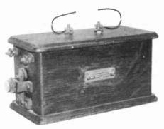
MANHATTAN SPARK COIL - This piece of wireless gear was produced in 1915 by the Manhattan Electric Supply Co. of Chicago and New York. The oak case is 81/2" x 41/2", and it has a 11/2" spark gap. (Wally Worth - Wollaston, MA)
