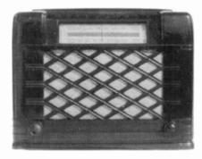
SILVERTONE MODEL 7100 – This 1942 set is battery-operated using 4 tubes: 1A7, 1A5, 1N5, and 1H5 octal base. This radio uses permeability tuning instead of the usual ganged tuning capacitor. The interesting thing about this set is the use of plug-in adaptors to utilize a 1S5 miniature tube to replace the 1A7. A coat of brown shoe polish and a rub with 0000 steelwool brought the Bakelite finish back to a new lustre. (Robert Pote – Greenwood, IN)
