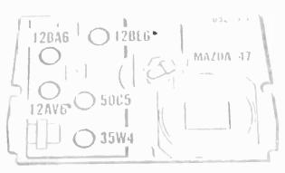
Figure 4. A tube and dial lamp layout is conveniently located on a label on the bottom of the set along with the suggestion: "For finest performance use only genuine RCA radio tubes."
