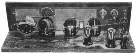
Figure 2. This interior view of the 2-tuber shows the spacious layout and some very long runs of bus-bar wiring.
