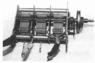
Figure 1. The tuning capacitor used in the Pilot radio.
