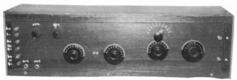
Figure 1. This example of an early home brew is a 2-tube regenerative set enclosed in a wooden cabinet about 21/2 feet wide. The panel, also made of wood, is hand-lettered in white paint.
