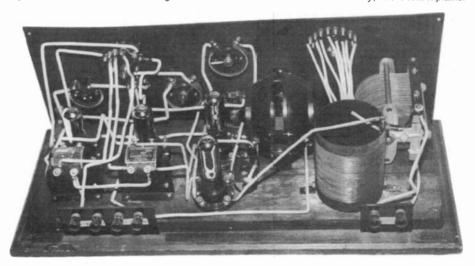
Figure 6. The 4-dialer was wired with white rubber-coated copper wire.
