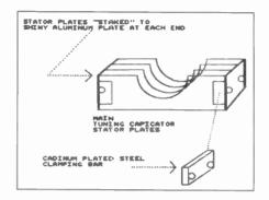
Figure 2. Tuning capacitor stator plate detail.
