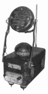
SEARS AUTO RADIO – This DC-powered receiver was actually built for operation on a farm tractor. (Clark Trissell – Lincoln, NE)
