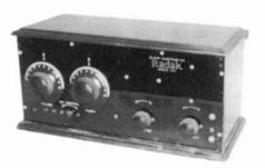
RADAK MODEL DD - This 3-tube receiver was manufactured by the Clapp-Eastham Company of Cambridge, Mass., in 1925. The cabinet measures 15<sup>3</sup>/<sub>8</sub>" long by 7<sup>1</sup>/<sub>2</sub>" tall. In addition to this wooden version, a leatherette version was also produced. (Wally Worth – Wollaston, MA)
