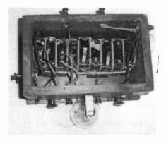
Figure 6. The 9 small batteries of the De Forest JR-4 are exposed because the bottom of the JR-4 was missing.
