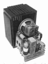
a resistance cord with a red jeweled pilot light. The right metal dial escutcheon is calibrated at 0-100, which is odd for 1934. The 2 knobs and nameplate are missing. (Ralph Jackson – Northboro, MA)
