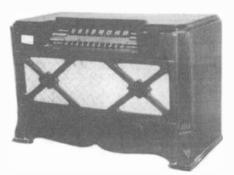
FARNSWORTH MODEL ET-066 – This 1946 fancy, wood cabinet is 9" tall and 24" wide. The dial scale is "Broadcast" (top) and "Log Scale" (bottom). The set has 6 tubes. (Wally Worth – Wollaston, MA)
