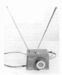
CHANNEL KING ANTENNA – This early 1950s adjustable TV antenna has a plastic base. The large knob adjusts the thin, flat, metal arms up or down. (*Alton A. DuBois, Jr. – Queensbury, NY*)
