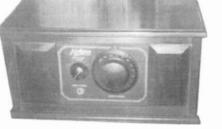
The "shortwave attachment" is a 1-tube 1920s Airline battery operated radio.
