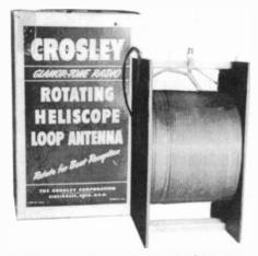
CROSLEY ROTATING HELISCOPE AN-TENNA – This loop antenna was recently purchased at a local auction. It has a connection for an outside long-wire antenna with 3 lead wires. It is then rotated for better reception. The box is 7" x 7" x 12". (Everett Hoard – Lehr, ND)
