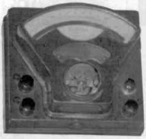
WESTON MODEL 1DC VOLTMETER - The cover of this instrument appears to be copper, and it is painted red. The last patent date is July 16, 1901. (Joseph G. Jackson - Macon, GA)
