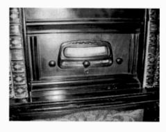
Figure 5. A view of the control panel of the Victor RE-75. The tuning knob is set at its midposition.
