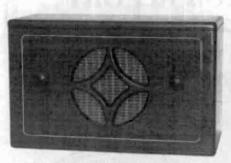
AMERICAN BOSCH MODEL 5 - This 1935 TRF uses two Type 24 tubes as RF amps, another Type 24 as a detector, a Type 47 for output, and a Type 80 as a rectifier. The tuning, which is not very selective, is done by direct drive with a very small window escutcheon. The cabinet and chassis are neatly done. (George Hausske - Wheaton, IL)
