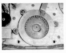
Figure 2. The lever-actuated cam-wheel, trimming rollers and trimming screws. The trimming screws were adjusted at the factory for best racking.
