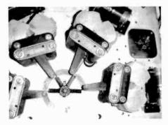
Figure 3. An under-chassis view of the tuning capacitors fully opened and their actuating mechanisms. The hex nut at the center is the stationary pivot.
