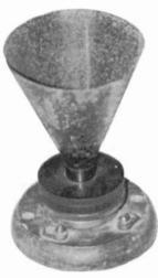
MICROPHONE OR SPEAKER, UNKNOWN – Neither the manufacturer nor the model number of this piece is known. Its construction is similar to an earphone driver with a magnetic coil and metal diaphragm. Is it a type of microphone or an inexpensive type of horn speaker? (Joseph G. Jackson – Macon, GA)
