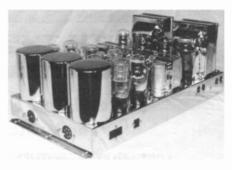
Figure 5. The 12-tube power amplifier chassis.
