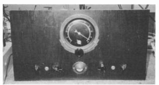
Figure 2. Ed Sheldon's Miller tuner. Note the tuning eye tube at the bottom center. Unlike Dick Parks' tuner that is calibrated in kHz, this tuner has an airplane-type dial calibrated from 0 to 100.
