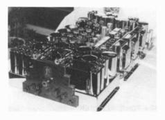
Figure 1. The completed 48-tube set. The four chassis can be seen with the tuner in front.
