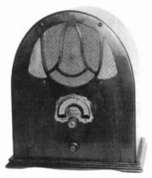
CLARION MODEL AC-100 - This 6-tube superhet cathedral was manufactured by the Transformer Corp. of America. It uses the following tubes: (2) Type 24; (2) Type 51; (1) Type 47; and (1) Type 80. The dial light moves with the pointer. (George E. Hausske - Wheaton, IL)
