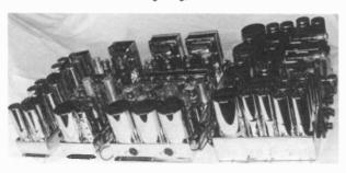
Figure 2. The four chassis can be seen clearly in this view from right to left: the 19-tube tuner, the 12-tube power amplifier, the 7-tube recording amplifier and the 8-tube crossover.
