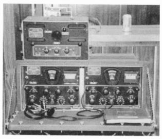
A Navy semi-portable RBM-4 receiver set owned by Paul Thekan, N6FEG. Two storage batteries for primary power are below the carrying case/table. The set of 2 receivers weighs about 350 pounds and covers 200 kHz to 20 MHz. The top control unit allows operation of either receiver at one time or both receivers simultaneously.
