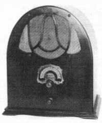
CLARION SERIES 100 - This superhet of 1932 vintage uses Type 51 tubes as RF and IF amps, Type 24 as mixer and 2nd detector, Type 47 or PZ for output, and the usual Type 80 as a rectifier. It was made for 60- or 25-cycle operation. See Rider's Volume II for a diagram. (George Hausske - Wheaton, IL)
