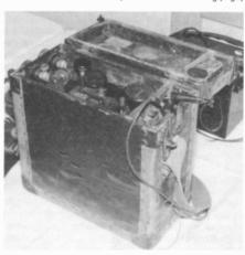
This SCR-74 military transmitter, a blue ribbon winner, has an unusual feature — the telegraph key knob protrudes through the lid so that the transmitter can be operated with the lid closed.
