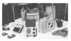
A variety of portable radios including the 1946 tube-type, suitcase look-alike "Sporter," right center, and several 1960s transistor radios, left.
