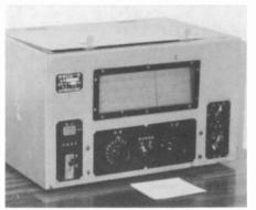
This Japanese "morale receiver" was built in 1943 and has 9 tubes. It operates on the broadcast band and 6-18 MHz. It is owned and operated by Ludwell Sibley, KB2EVN.
