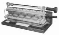
SPARK GAP, MANUFACTURER UNKNOWN – This adjustable spark gap, ca. 1918, has 10 spark gaps in series. It is set on a walnut base with a vertical glass shield in front. The large knob adjusts the gap distance, while the smaller lower lever puts the gaps in service. (Wally Worth – Wollaston, MA)
