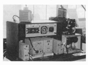
ed points, while the other two are called "Outer" or "Middle" markers (OM/MM). The OM and MM transmitter sets are located on the flight path to the runway for landing purposes. The transmitters are modulated with three different audio tones to activate the lamps.
