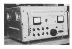
A Rhodes and Schwartz Model EK-07D German receiver owned by Dan Arney, KN7DI. Sometimes referred to as the "Rolls Royce R-390," this receiver was in the \$5,000 range in the early years of its production. The 27 tubes can be checked in circuit by a built-in test meter. The weight is 150 pounds and the frequency range is 500 kHz to 30.1 MHz.
