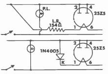
Figure 2. These "Before" (top) and "After" (bottom) schematic diagrams show the use of a solidstate rectifier as a resistance line cord substitute.
