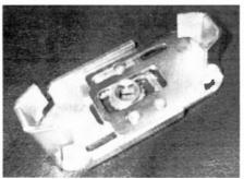
Figure 1. The Sears oil filter wrench.
