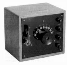
K & C CRYSTAL SET – This simple 1922 crystal radio is built into a 5" square oak box and was manufactured by Kilbourne & Clark of Seattle, Washington. (Byron Wingett – Anacortes, WA)
