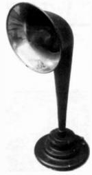
TMC HORN SPEAKER – This small metal horn with wooden base was made in England by the Telephone Mfg. Co. TMC on the nameplate is defined as "TrueMusiC." It is 18" tall with a 6" wide bell that is electroplated copper inside. (Dave Crocker – Mashpee, MA)
