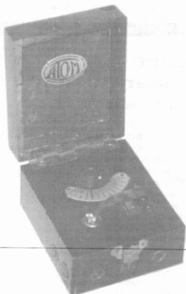
ATOM CRYSTAL SET – This relatively small set was made by Radio-Merkur, a Vienna factory about which not very much is known. The catwhisker is a flat, tapered piece of metal. (Erwin Macho – Vienna, Austria)
