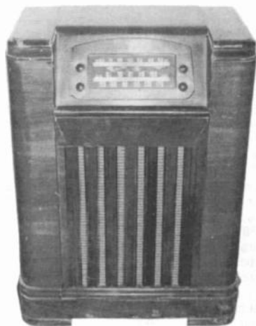
PHILCO MODEL 46-1226 – This 1946 console radio features a pull-out phonograph just below the dial face. The entire front grille section is hinged at the bottom. It tunes the broadcast band, as well as the shortwave bands. (Clark Trissell – Lincoln, NE)
