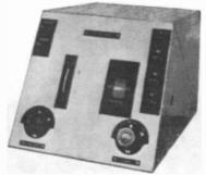
Figure 2. Front panel view of the 1st RF stage with its cover in place. The antenna and ground binding posts are located on the top left corner of the unit. The binding posts on the right make electrical connections to the 2nd RF stage. The thumbwheel dial, center left, is mechanically linked to the tuning dial, center right, and the variable capacitor. The antenna coupling switch is located at the bottom left, and the filament rheostat to control RF gain is located at the bottom right.
