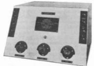
Figure 8. The radio's nameplate is mounted on the front panel of the audio amplifier unit. The controls at the bottom are filament rheostats.
