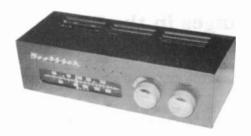
HEATH MODEL BC-1A - This 1959, 5-tube, transformer-powered, broadcast tuner is capable of a flat response to 9 kHz. When it receives AM stations using wide range programming, the effect is similar to FM. A bridged-T filter is employed to reduce the annoying 10 kHz beat note prevalent on the AM band. Two outputs are available from phone jacks, one medium impedance, fixed, and one low impedance, variable. (Roland Jenkins - Leavenworth, KS)
