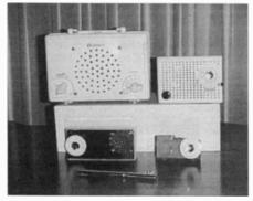
Figure 3. The Philmore TR-22 transistor radios (top) are shown in contrast to the smaller versions Ralph built himself.
