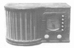
ZENITH MODEL 5R317 – This is Zenith's "Glass Rod" radio of 1938. Purchased at a second-hand store for \$35, it needed restoration. I replaced three of the glass rods and had repro push buttons installed. It is now in working condition. (James Apthorpe – Leesburg, FL)
