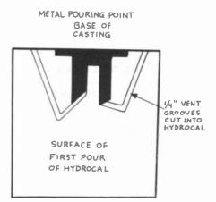
Figure 5. It is necessary to cut paths in the mold to allow air to escape when the molten metal is poured into the mold.
