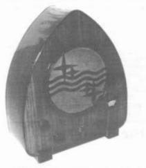
PHILIPS MODEL 930A – This 4-tube AC (mains) cathedral receiver was manufactured in London in 1930. The wood-grained cabinet is of Arbolite laminate. (*Jim Taylor – Bournemouth, England*)
