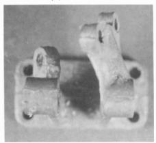
Figure 1. A top view of the original pot metal casting after the dial cord pulleys and shafts were removed. Note the cracked arms and angles of the arms.
