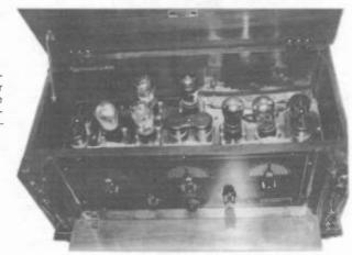
DAVID GRIMES MODEL 6D – This 1926, 6-tube receiver features binocular coils. The cabinet has a pull-down, frontpanel lid. (*Wally Worth* – *Wollaston, MA*)
