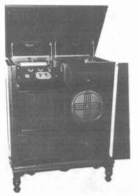
BRUNSWICK MODEL PR-138C – This radiophonograph combination console, called the "Panatrope," was Brunswick's top-of-the-line offering in 1926. The set consists of an RCA Radiola 28 receiver having 8 tubes, a Brunswick 78 rpm phonograph, and a built-in speaker. The AC version sold for \$995, while the DC version sold for \$945. (Donald S. Cockrane – S. San Francisco, CA)
