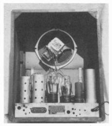
Figure 2. The rear view of the Wilcox-Gay radio showing the chassis, tubes, speaker and, at the bottom, the location of the jumper jack for either radio or phonograph operation.
