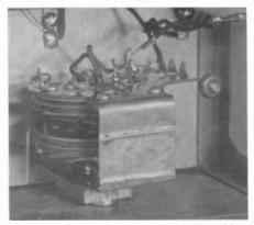
Figure 2. The repaired antenna coil assembly.
