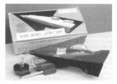
GLOBE MODEL MG-308 – This highly stylized rocket ship is a germanium crystal radio that tunes with a rod in the ship's nose. It was manufactured by the Globe/Miniman Radio Co. of Japan. (*Harry Blesy – Hindsdale, IL*)
