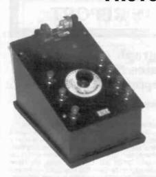
**EUMIG CRYSTAL SET** – This is one of the earliest sets from the Eumig factory in Vienna. It was built in 1924 and has slide tuning. The plug-in crystal detector is labeled "King." (*Erwin Macho – Vienna, Austria*)
