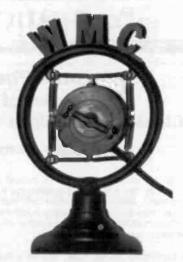
WESTERN ELECTRIC MODEL 387W MICROPHONE – This 1920s double-carbon, spring-type microphone was used in the early days of broadcasting. Radio station WMC celebrated its 75th year on the air in 1998. I worked for the WMC station for 35 years and retired in 1997. (Willis Rudolph – Memphis, TN)
