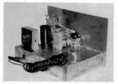
Figure 6. The Multivalve Receiver No. 3 superheterodyne, using a Type 6AS11 Compactron.
