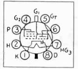
Figure 1. The base diagram for the Type 6M8GT tube.
