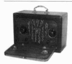
SPARTON MODEL N-61 – This tiny, 1933, 5-tube radio, only 7" tall and 9¾" wide, is housed in a cherry wood case with pull-down front. The decorative handle on top is made of brass. (Wally Worth – Wollaston, MA)
