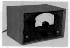
Figure 7. A 2-band version of the 1-tube superheterodyne, using plug-in coils.
