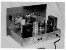
Figure 5. The Multivalve Receiver No. 2, using a Type 14BR11 Compactron in a straight TRF circuit.
