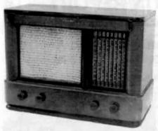
PHILCO TROPIC, MODEL 42-761 – This set appears to be from the same family of radios made for New Zealand distribution. It has permeability tuning and 8 separate broadcast bands. Found in an old storage trailer in a salvage yard, it is in remarkably good condition. (Barry Siembor – Woodinville, WA)
