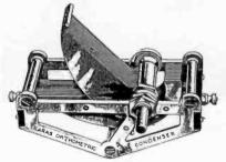
Figure 4. A typical variable tuning condenser used by many radio manufacturers.
