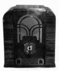
ERLA MODEL 5728E - This 5-tube Erla tombstone has the following tube complement: 2A5, 2A6, 2A7, 58 and 80 rectifier. The small dial is in three colors: green, red and ivory. The dial face, not the pointer, rotates. This is a 3-band receiver. (Victor Marett - Miami, FL)
