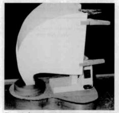
Figure 3. Side view of the cardboard templates for the horn bell held to shape by clothespins. Note the temporary support bracket at the front of the horn.
