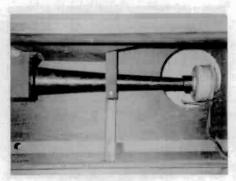
Figure 2. The radio removed, exposing the Atmater Kent hom and driver. Surely that thing will unscrew easily?
