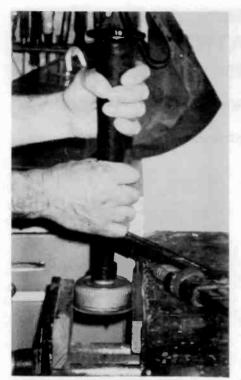
Figure 3. The milled edge of the ariver base held in soft wood, but nothing budges.
