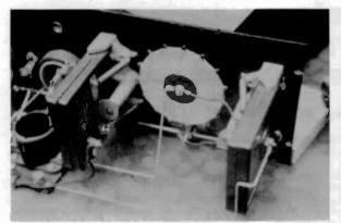
Figure 5. This photo shows how the Crosley book condensers are mounted on the back of a typical radio panel.
