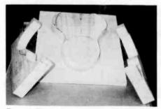
Figure 1. The wooden, violin-shaped forms. The center section is screwed to the bottom board for stability during work.
