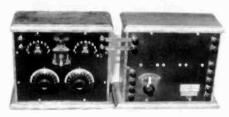
W.W. GRANT CRYSTAL SET – The crystal detector used on this receiver is a Freshman double adjustable unit. The receiver is connected to a Northern Electric Type 106 amplifier which uses (2) Type 216A tubes. (Paul Luehr – Alberta, Canada)
