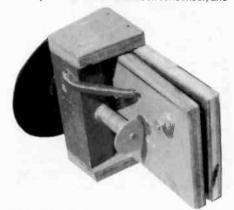
Figure 2. Powel Crosley's first book-type tuning condenser, the Type A, used in his early model receivers, was constructed mostly of wood.
