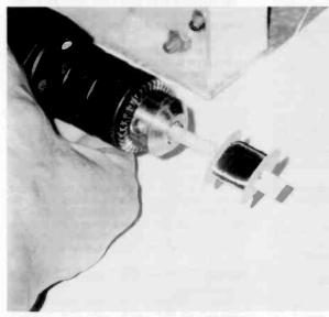
Figure 6. Rewinding the open coil on a homemade bobbin.
