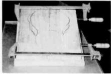
Figure 2. The sections of the wooden form are clamped together to hold the veneer to the desired shape during the setting of the glue.
