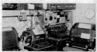
Figure 8. A view of the RTTY comer of the Ham shack. These old mechanical teletype machines were noisy and required much maintenance, but they were fun to operate.
