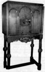
ZENITH MODEL 35 PX - I recently finished a total restoration of this 7-tube TRF console. It was purchased new by the previous owner in 1925. When the restoration was completed, the set worked beautifully, picking up stations all over the country. (Alan McFarlane - Aberdeen, SD)
