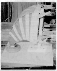
Figure 5. The wooden veneer pieces, taped into position while the glue dries, form the hom.
