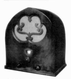
DWARF CATHEDRAL – This 4-tube superheterodyne radio was manufactured in 1931 by the Dwarf Radio Mfg. Co., located at 6725 Santa Monica Blvd., Hollywood, California. (Kenneth Acord – Long Beach, CA)
