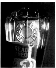
Figure 1. The brand name "Raytheon" is stamped on the metal plate inside this Type ER201A vacuum tube.
