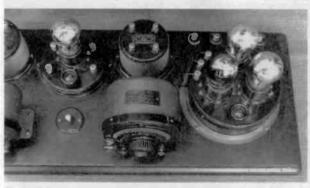
Figure 6. A view showing the multiple use of binding posts on the components on the right side of the Radiodyne receiver.
