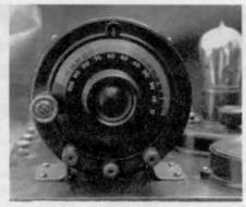
Figure 8. One of the Radiodyne tuning condensers showing the binding posts at the bottom.
