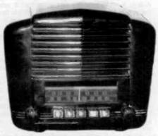
CROSLEY MODEL 628-B - This 1937 Bakellte radio has a broadcast and shortwave band which tunes up to 7.0 MHz. It has a 6-tube, AC powered chassis utilizing a 2W3 half-wave rectifier. It is a fine example of the Decostyling of the late 1930s. (William Dalton, Jr. - Bridgeport, CT)
