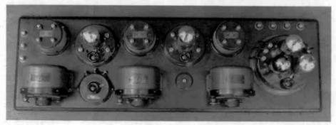
Figure 2. Top view showing the placement of the Atwater Kent breadboard components on the Radiodyne receiver.
