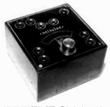
MINIM CRYSTAL SET – This simple crystal receiver may be of Scandinavian manufacture. The logo design is difficult to read, quite possibly "Teta." The panel has jacks for two antennas and two headphone inputs. (Erwin Macho – Vienna, Austria)
