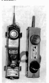
6 VHF FM unit on the left and the WW-2 BC-611 on the right. The BC-611 operates on the 80meter band with AM modulation.
