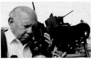
Forest Ogan, W7VQH, calling for assistance on 51 Mc FM after running into a tank. The battery operated HT is a single channel PRC-6 that puts out about 1/2 watt of RF.
