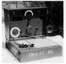
The BC-148, dating back to 1930, was still in use ten years later. This one has a 1940 date on the name plate. The 1-tube transmitter and 3-tube receiver use a loop antenna for CW work out to about 5 miles. Output is about 5 watts. Operating instructions and schematic are to the right of the key.
