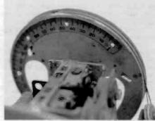
Figure 6. The protractor scale attached to the back of the dial pulley for the alignment procedure.
