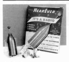
**HEAREVER MODEL 20** – This rocket-shaped, germanium crystal radio tunes by moving the nose rod on the front of the rocket. The claim on the front of the original box says: "Still The World's First Radio." (Harry Blesy – Hindsdale, IL)
