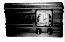
ROGERS MODEL 15/50W - This compact design in a small wooden cabinet was made in Toronto, Canada, in 1940 by the Rogers Majestic Corp., Ltd. The 5-tube AC chassis uses the following tubes: 12A8MT, 12K7MT, 12B6MT, 35L6GT and 50Y6GT. The radio features slug luning, series filaments and full-wave rectification with plate transformer. The electrodynamic speaker field serves as a filter choke. (Orval Egeter - Fonthill, Ontario, Canada)
