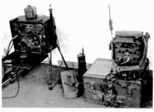
A U.S. Navy TBY set on display at right with a U.S. Army BC-611 HT at left. The CRI-43044 transceiver operates from about 28 Mc to 80 Mc for short distance work. Output on CW is about 3/4-watt and 1/2-watt on phone. At far left, is an Army SCR-284 field set.
