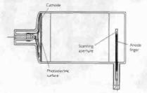
Farnsworth's camera tube, from "Tube: The Invention of Television," p. 129.
