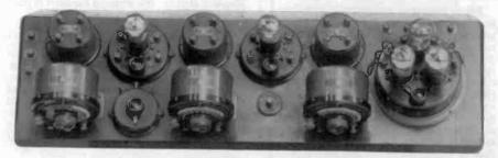
ATWATER KENT MODEL 10 - PART NUMBER 4340: Model 10 was the most common of the bread-boards. Number 4340 was the first of four major variations of Model 10. The set had three radio frequency resonators. The coils were parallel with their axes vertical. The tuning condensers were green in color as was the three-tube unit. Nameplates and binding post were used to connect the coils and the condensers in the first sets produced. The size of the base board is 31½ x 10 inches.
