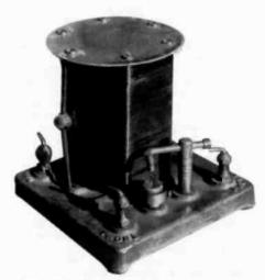
MARTIAN SPECIAL – This crystal set is the "little brother" to the Martian Big 4 tripod crystal receiver. It is also related to the unique 1-tube Martian Beauty, all produced by the Martian Radio Company of New Jersey. This "Special" has a cast metal base and the distinctive Martian L-shaped binding post caps. It has a single sliding ball tuner at one side of the coil. (Dave Crocker – Mashpee MA)
