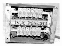
Figure 3. Bottom view showing the bank of push button trimmers.
