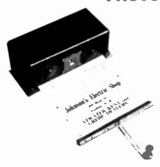
TOY ADVERTISING RADIO – This novelty radio is approximately 4" x 2" x 11/2". It is made of black, wrinkle-finish, painted tin. The attached string unrolls a long fabric roll with station dial locations on one side and a weekly programming log on the back. No manufacturer's name can be found on the radio; however, it advertises "Johnson's Electric Shop in Nashua, New Hampshire." Pulling the roll outwards also changes the numbers behind the small brass dial escutcheon. (Dave Crocker – Mashpee, MA)
