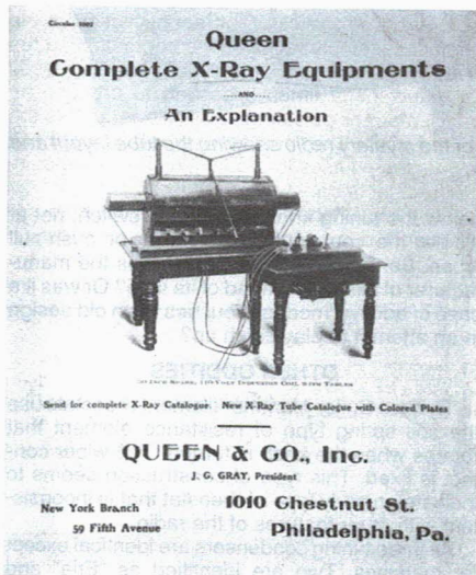
This Queen & Co. cover of a turn-of-the century catalog illustrates a 30-inch spark set-up for use with x-ray equipment.
