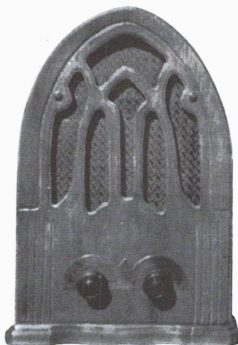
MAJESTIC MODEL 194 – This little 4-tube cathedral, made in 1933, performs well on the broadcast band, even without an antenna! The shortwave switch is on the back of the chassis. Shortwave reception is OK, but of course it needs an antenna for the best reception. ( Ben Martin – Castro Valley, CA )
