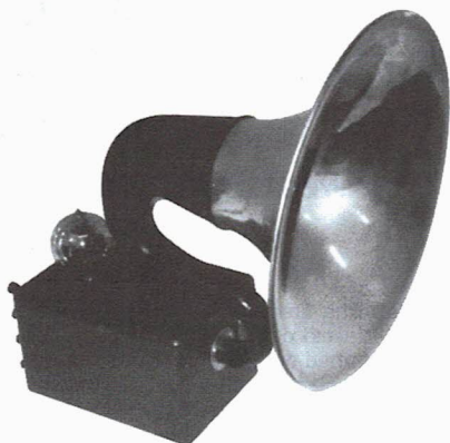
CLEARTONE HORN SPEAKER – Made by Cleartone Radio Co., Cincinnati, Ohio, this speaker has a 1-stage amplifier built into its base. The nickel-plated bell is 11" at the mouth and 15" high. ( Ed Bell – Raleigh, NC )
