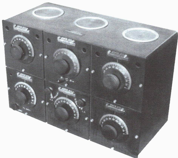
AMRAD TYPE 3500-U RECEIVER — This double-decker was one of the last of the multi-level combination receivers made by the American Radio and Research Corp. of Medford Hillside, Mass. The set consists of six separate units. From left to right, on the top row, the units consist of: (1) Type 2771 VT detector and (2) Type 2766 VT 1-stage amplifiers. The panels in the bottom row, left to right consist of: (1) Type 3290 RF 1-stage amplifier, (1) Type 2753 variocoupler and (1) secondary. It is a 4-tube receiver, each tube section having a screen cover. The fourth screen cover is on the left side of the cabinet panel of the Type 3290 RF amplifier. The 3500-U has a total of seven metal nameplates. (Dave Crocker — Mashpee, MA)
