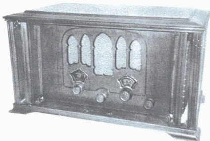
GENERAL ELECTRIC MODEL GE K-51 — The ornate "carved" doors on this 1932 wood table model open and slide into the ends of the cabinet. The radio features broadcast plus police band. (Don Howland — Spokane, WA)
