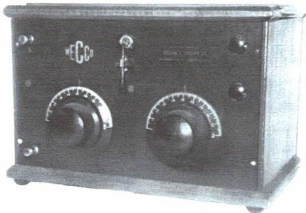
WECCO CRYSTAL SET – This 1925 Stowell model, made by the William E. Cheever Co., 90 Arlington St., Edgewood, Rhode Island, has a top lid that opens for access. The dimensions are 7 \frac{1}{4} " x 10 \frac{3}{4} " x 6 \frac{3}{4} ". ( Ed Bell – Raleigh, NC )
