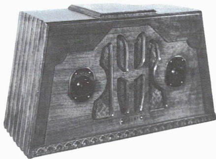
WARWICK MODEL 45, SERIAL #10046 – Warwick Mfg. Co., Chicago, Ill., produced this Art Deco model, ca. 1933. It is in original, mint condition, including a wooden back. This AC/DC TRF set uses a resistance line cord with 4 tubes — Types 12Z3, 43, 6D6, and 6C6. (Rod Kennedy – Morago, CA)
