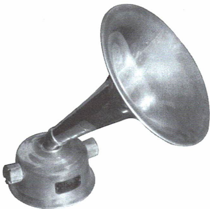
MOON HORN SPEAKER – This all aluminum, headphone-driven speaker was produced in Dayton, Ohio, by the Wilson Utensil Company, which also manufactured a line of pots and pans. Headphones fit over the two rubber pads, and the horn neck can swivel completely around. (Dave Crocker – Mashpee, MA)
