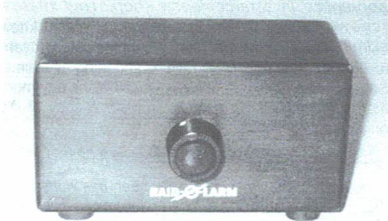
Figure 1. The tiny Raid-O-Larm cabinet, measuring only 6" x 3" x 3".
