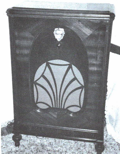
Figure 6. This 1930 A.W.A. Radiola Model C64 console performed well for a 6-tube TRF. The 1-dialer made radio far more accessible.
