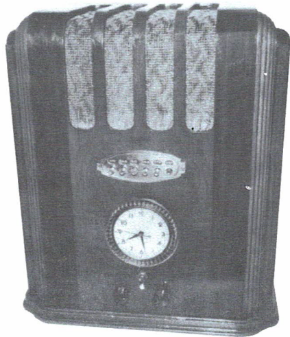
SPARTON MODEL UNKNOWN — This interesting and unusual 1937 Sparton tombstone radio has neither dial nor tuning capacitor. Tuning is done with the six push buttons located just above the clock dial. The radio can be turned on manually or automatically with the built-in timer. The white dot between the knobs is the pilot light. A socket in the chassis will accept a Type 6E5 tube to help in setting up the push buttons. Please contact A.R.C. if you know the model number of this truly unique set. (W. R. Cobb – Laguna Hills, CA)
