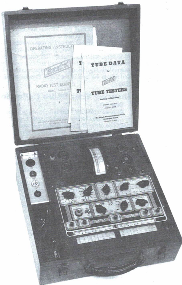
Figure 4. AC51 (1935), the first model to use the "Hickok" (Barnhart) circuit. The edgewise meter saved panel space. The auxiliary socket panel was built from plans in the data booklet pictured, probably in the late 1940s.
