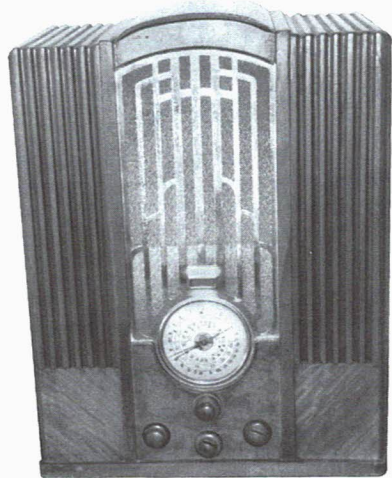
ZENITH MODEL 935 – This ca. 1935 Art Deco tombstone is very similar to the Model 835 shown in Alan Jesperson's book on Zenith radios. I understand it was pictured in the Time-Life series on collectables. The set has five bands, shadow meter and 10 tubes. (John C. Baldwin – Makawao, Maui, HI)
