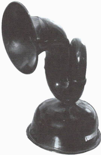
ARKAY HORN SPEAKER – This black lacquer over brass horn speaker was manufactured by the Riley-Klotz Co. of Newark, New Jersey. Under the base is a clamp which holds a Baldwin driver unit in place. (Dave Crocker – Mashpee, MA)
