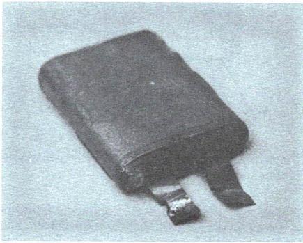
Figure 6. An example of an early paper dielectric capacitor in a flat-wound configuration.
